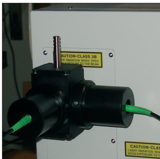
Fig. 1: Polarization extension mounted at the exit port of an Olympus Fluoview FV1000 scan head.
